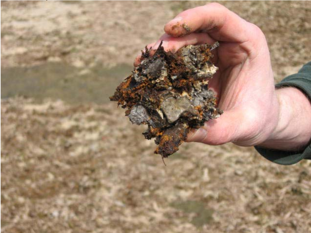
Photo 3. Materials cemented by metals solids at the top of the Big VFP organic substrate layer
