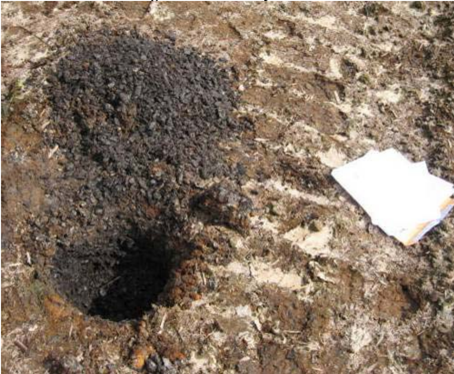
Photo 1. Small VFP organic substrate layer contents
