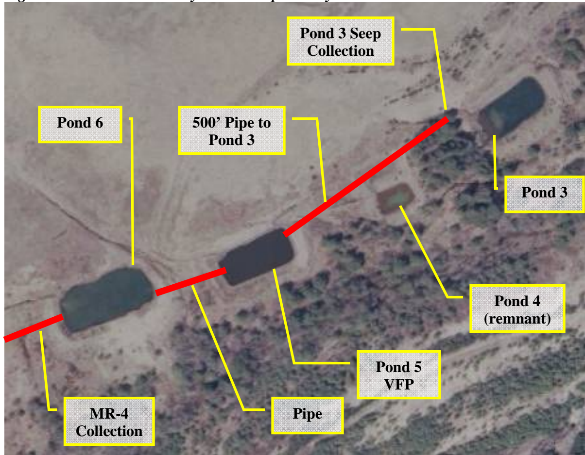
Figure 3. MR-4 Treatment System Conceptual Layout
