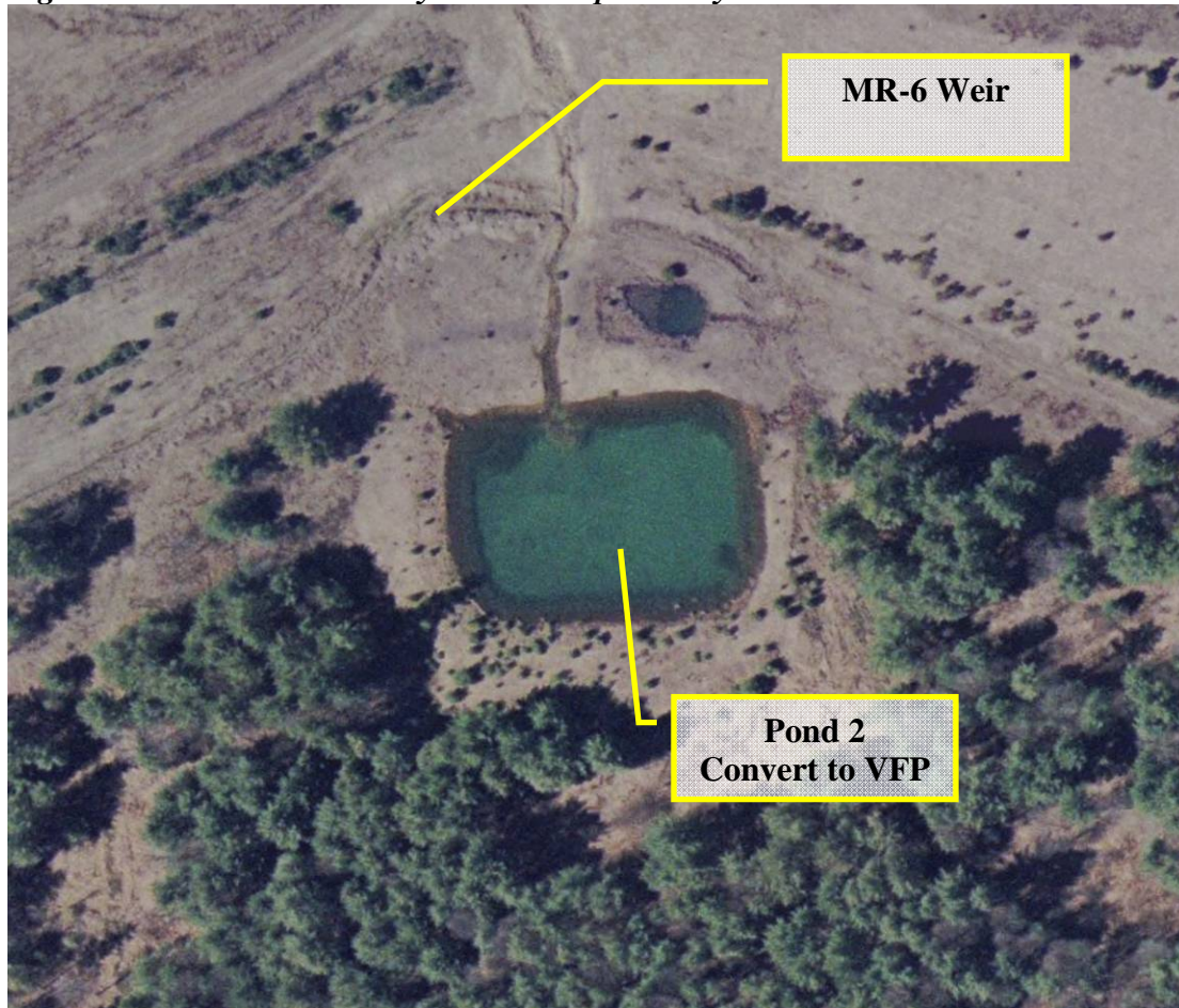
Figure 4. MR-6 Treatment System Conceptual Layout
