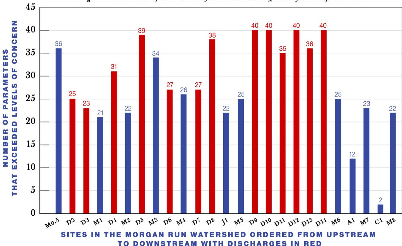
Hardness was approximated by taking a regression of measured calcium and magnesium values with data from other subbasin surveys. This analysis indicated that aquatic life tolerance levels of concern for manganese were exceeded at D7, D8, D9, D10, D11, D12, D13, and D14 rather consistently in each quarter of sampling. This suggests that a priority area for manganese pollution remediation should be the discharges in SGL #98.
