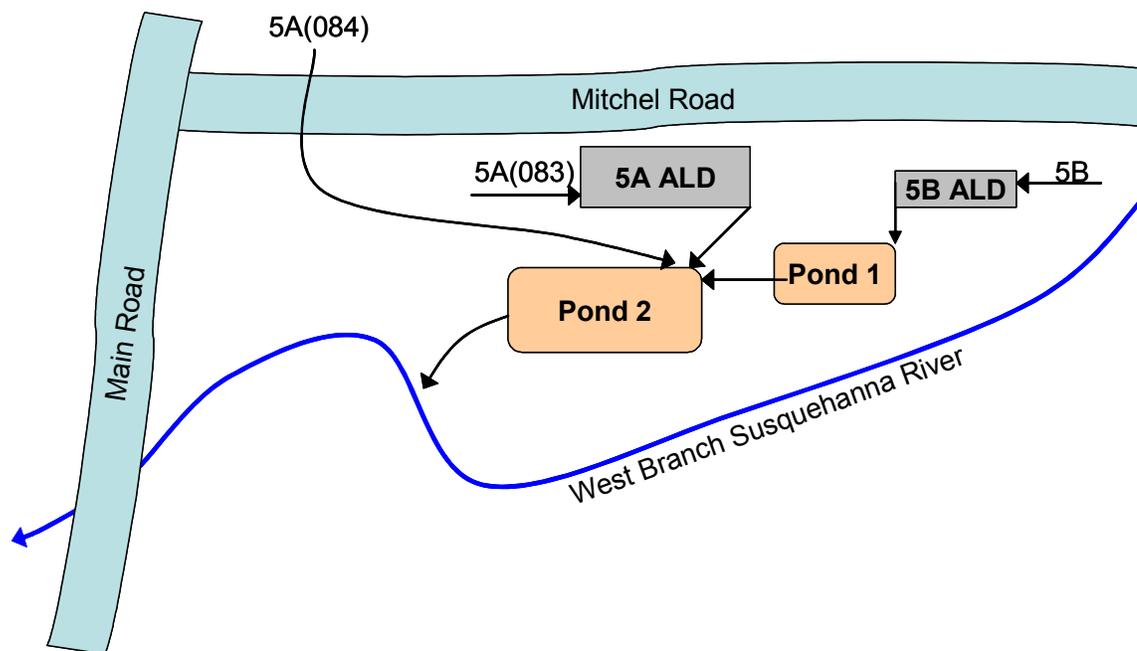
Two small ALDs should be constructed. The 5A(083) discharge requires 600 tons of limestone and the 5B discharge requires 330 tons of limestone. This quantity of limestone will provide sufficient treatment of the discharges for at least 25 years before more limestone needs to be added. Construction of the ALDs will require collection of the two diffuse seep zones in French drains. The water will then flow to the buried ALDs.
